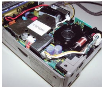
OS-CON is used 10V/47 \mu FX2P size: \phi 6.3×L5.0
